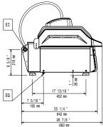
Electrical inlet (power) Electrical Outlet
